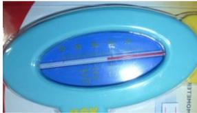
An alcohol thermometer can be used to measure the temperature of water of a bathtub to bathe a baby, or outside temperature.
